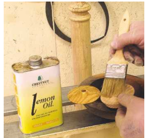
▲ Pic.33 The best matt finish for ash is lemon oil. The timber will need a couple of coats. Leave to dry and cut back with the Nyweb between applications
